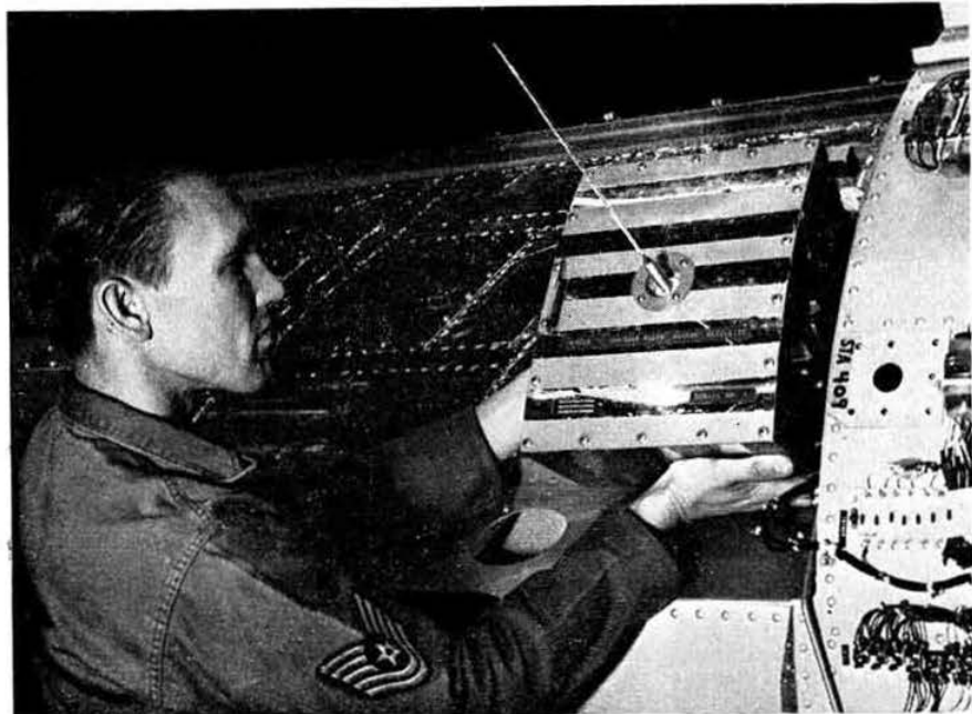
The Oscar I satellite being loaded on to the Discoverer 36 rocket at Vandenberg Air Force Base, California. The transmitter comprised a transistor crystal oscillator on 72.5 Mc/s, a transistor amplifier and a "Varicap" diode doubler to 145 Mc/s, with a power output to the 19 in. quarter wave monopole of about 100 milliwatts. The oscillator was keyed in the base circuit by a transistor multivibrator and counters with diode logic. Power was derived from mercury batteries and the complete unit measured 12 in. x 10 in. x 8 in. excluding the aerial shown in this picture. Reports indicate reliable reception up to a distance of about 1400 miles from the satellite path.
